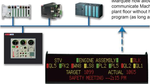
iMarquee now allows you to add a display to communicate Machine/Process status and alarms to plant floor without having to make any changes to PLC program (as long as the data is available in PLC).
