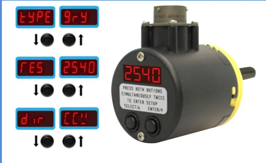
In addition to the ease of use and programmability in the field, the LED Display on the front of the Encoder provides immediate feedback to the user with the current position and speed (RPM) of the shaft during operation. As a side note, besides having one encoder fit all applications, the EZEncoders™ of Size 25 are also designed to be drop-in replacements for traditional BEI, Dynapar, Rockwell and EPC encoders.
