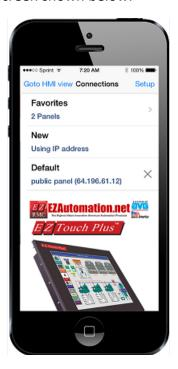
From this screen, you could select a panel to connect to. You can select a panel already saved in a Favorites list, or a New Panel by providing its IP Address, or to a Default panel, whose name and IP is given as Default.
