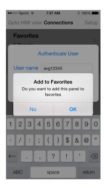
5. After selecting to add a panel to your favorites, you will be prompted to enter a name for the panel. Enter a label of your choosing. Also on this screen, you will have the option to save a password for accessing the panel or set the HMI as the default panel with the App using the slider. When finished press OK.
